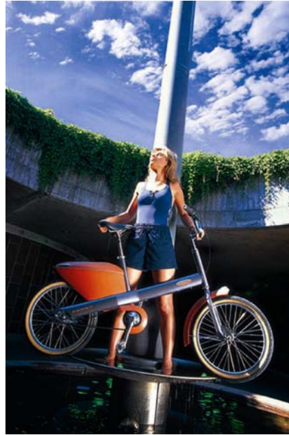
11. DBS' Komby. The luggage carrier also serves as a mudguard, a dress guard, a box that holds a fitting bag. The handlebar has an integrated compartment for mobile phones.
