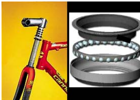
9. Cannondale road frame. By integrating the bearing system in the head tube, the conventional headset has been eliminated and the total weight reduced.
